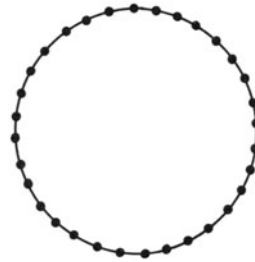
32 constant boundary elements 32 degrees of freedom (b) Boundary element model
